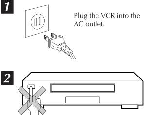
Don't press any buttons on the VCR or remote during auto setup.
