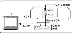
With this connection, you can view one scrambled cable channel while recording another unscrambled channel.
